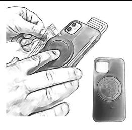
4. Hold down center of Mag Flex Plate with one hand and peel down and back the sides of position template. Double check you are centered and aligned than remove template. Press firmly with both hands the Mag Flex plate to your phone or case. Lets Adhesive cure for 10 minutes before use.
