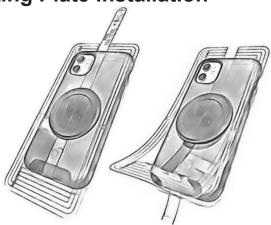
3. Point pull tab up and make sure Mob Armor Logo is positioned the direction you want it positioned. Peel down center tab to expose the adhesive center of Mag Flex Plate. Use letter and number markers to find the center of your phone over your wireless charging location.
